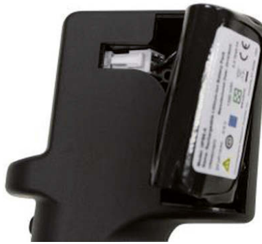
4. Push down on connector latch and pull battery loose from the board.
