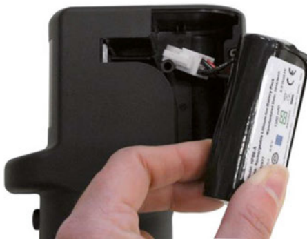
5. Connect new battery to board, making sure the latch is secure. Push battery into case, bending the wires if necessary.
